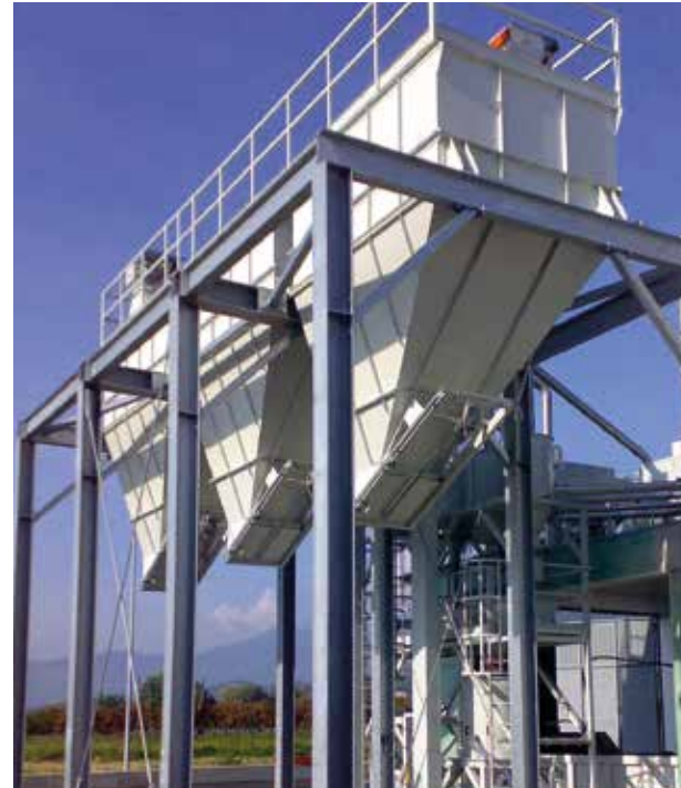
Silos a ponte Bridge silos Brückensilos
