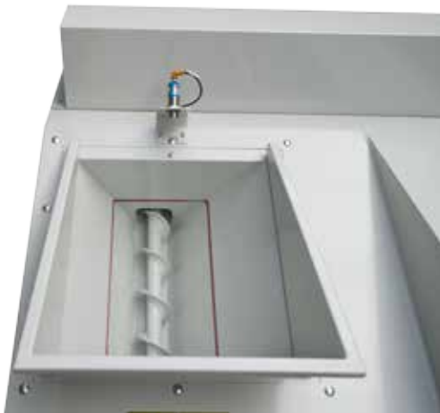
Material feed via screw. Filling by hand or automated. Illustration shows machine without container top and without intervention protection.
